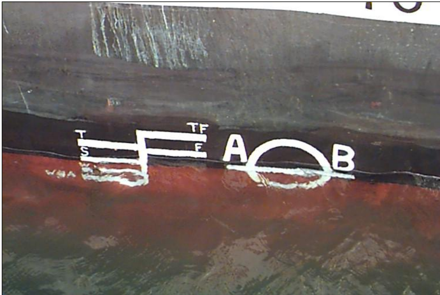
Figure 2. Plimsoll mark on the hull of a ship.
